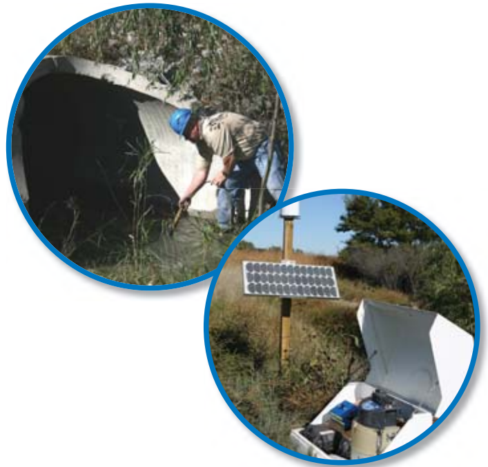
The 2105 system shown here interfaces a rain gauge, flow meters, automatic sampling, and a multiparameter sonde.
