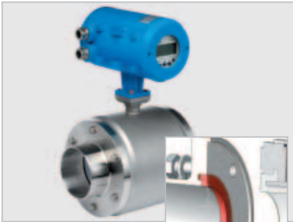
VARIFLUX 6000 compact design. Crevice-free seal between lined measuring tube and process pipe or adapter using L-shaped gasket with trapezoidal sealing lip
