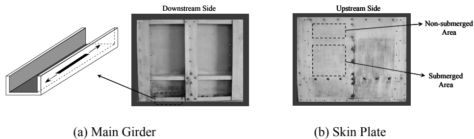
Figure 2: Sampling Methods of FRP Door Body for Tensile Test
