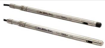
Conductivity measurements can be used to characterize water quality changes relative to a baseline or to estimate the concentration of contaminants. The In-Situ® Aqua TROLL 100 and Aqua TROLL 200 Instruments measure and log conductivity and temperature. The Aqua TROLL 200 adds water level logging.
