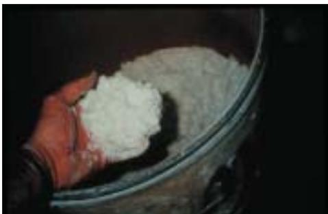
Fillers are used to enhance a specific property of a laminate, e.g. the addition of antimony trioxide to develop flame retardance, but they can also be used to bulk the resin with cheap filler at the expense of the finished laminate properties. It is important to assure that fillers are used wisely. In general, fillers detract from the performance of resin.
