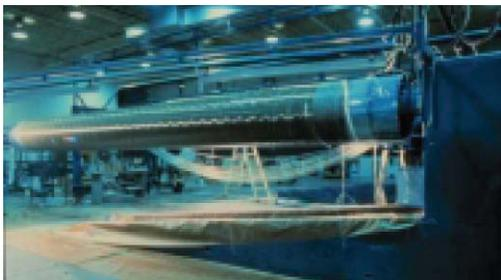
Although it is possible to wind complex structural shapes, filament winding in the corrosion industry is generally limited to cylindrical shells. It is used to produce small to very large diameter tank shells and straight pipe.
