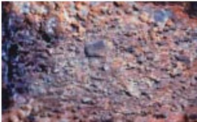
There are many corrosion mechanisms which affect ordinary carbon and low alloy steels, but by far the most common is that induced by the so-called oxygen cell, which occurs in the combined presence of acid, water, and air. Both hydrogen ions and molecular oxygen can function as electron acceptors to form an oxidation/reduction galvanic cell, and the steel functions as an anode to thereby become oxidized.
