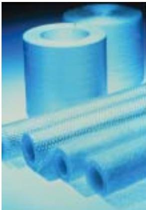
Fiber reinforcements that are used in the corrosion fiberglass industry include various forms of glass fiber, such as E-glass and a newer, more corrosion-resistant version, called ECR-glass. Synthetic fibers, such as polyester surfacing veil or carbon veil (for abrasion resistance and conductivity) are also available. Occasionally, aramid, or carbon fibers may be used in the structural laminates to improve the strength-to-weight ratio. The most common forms of glass reinforcement are:
